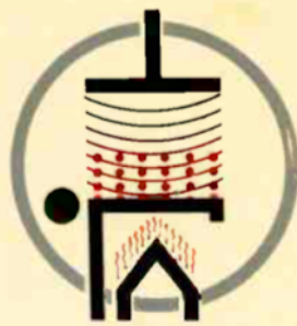
2. When it is negatively charged, the anode cannot attract electrons.
