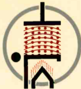
1. When it is positively charged, the anode attracts electrons.
