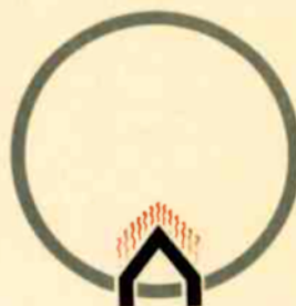
The heater heats the cathode
